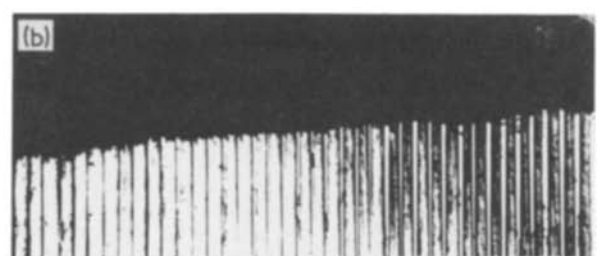
Figure 5 Micrographs of splitting zone for as-fabricated composites (a) B/Ti-6Al-4V, (b) SiC/Ti-6Al-4V.
